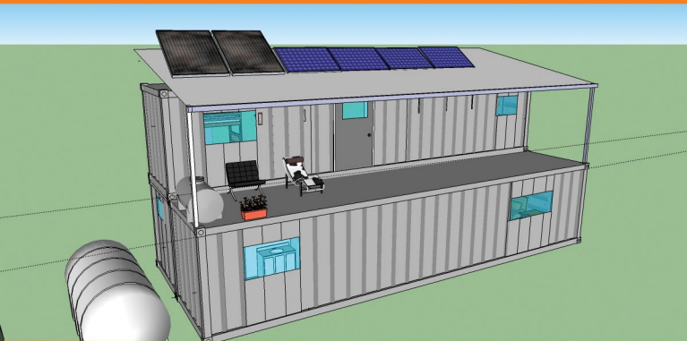
ROOF WITH PV AND HOT WATER SOLAR COLLECTORS
